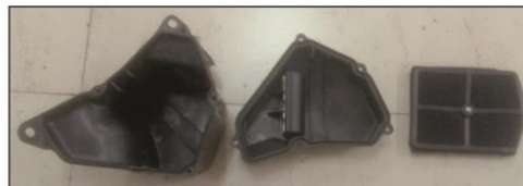
Removal of foam filter element
