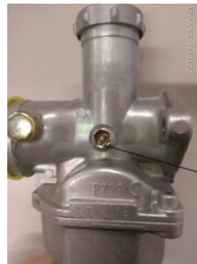
Idle Speed adjusting screw
