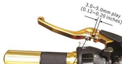
Clutch lever adjustment nut
