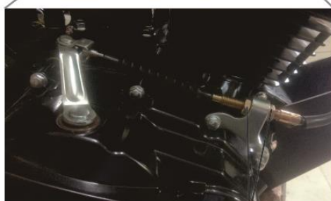
Clutch adjustment nut
