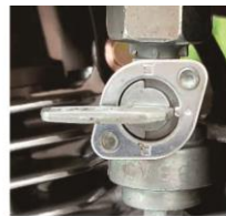
Fuel Valve OFF
